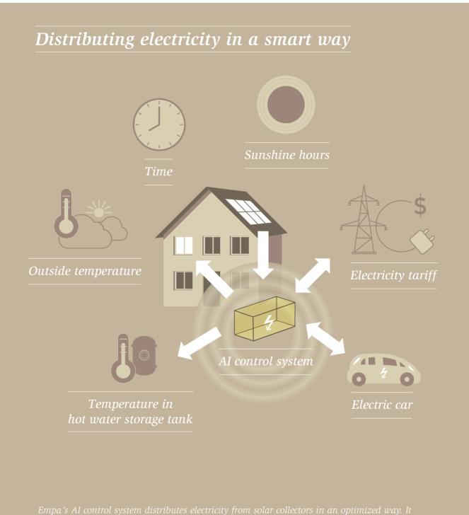
Empa's AI control system distributes electricity from solar collectors in an optimized way. It does not need to be programmed, but uses AI to "learn" the needs of the occupants and adapt to the time of day and season. It can be used for buildings of various types and sizes.
