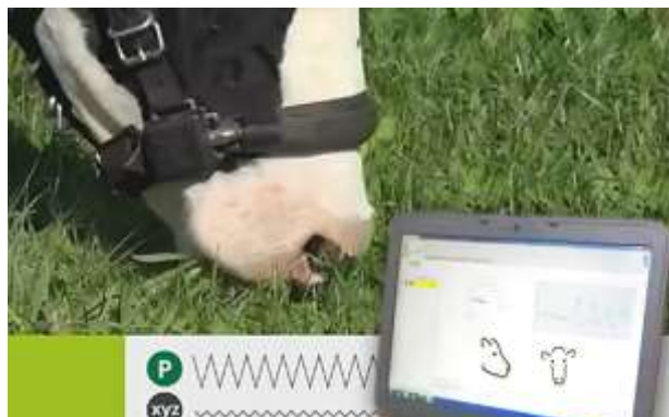
The RumiWatch system, which monitors the activity and health of dairy cows, is an example of Smart Farming.
