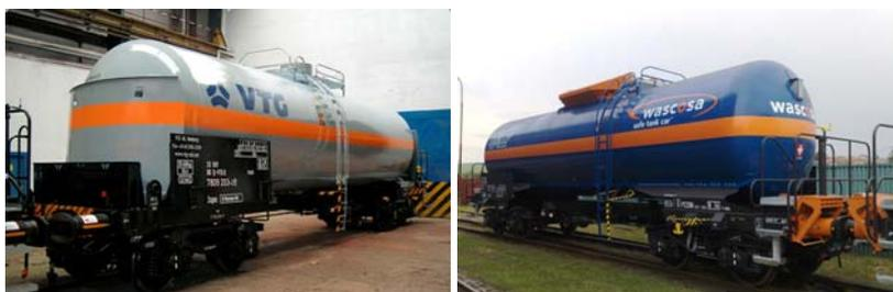
Figure 7 – Crash Protected Rail Tank Car (CPR II) de VTG et Safe Tank Car de Wascosa
