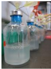
Image 1: Using so-called chemostats, bacterial cultures of Klebsiella oxytoca are supplied with varying concentrations of ammonium and an excess of gaseous nitrogen (N 2 ). (Copyright: Frank Schreiber)
