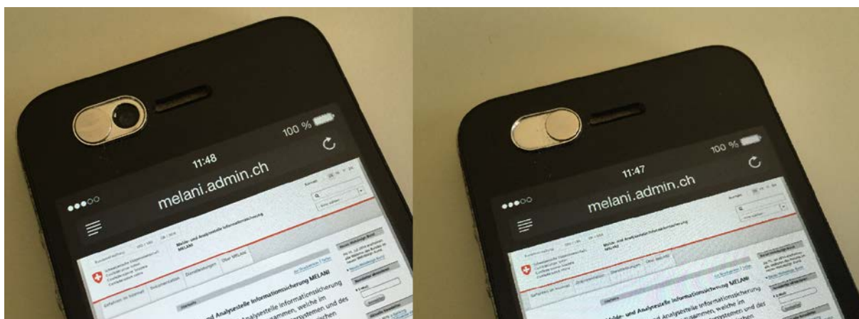
Figure 5: A temporary camera cover both open (left) and closed. 8
