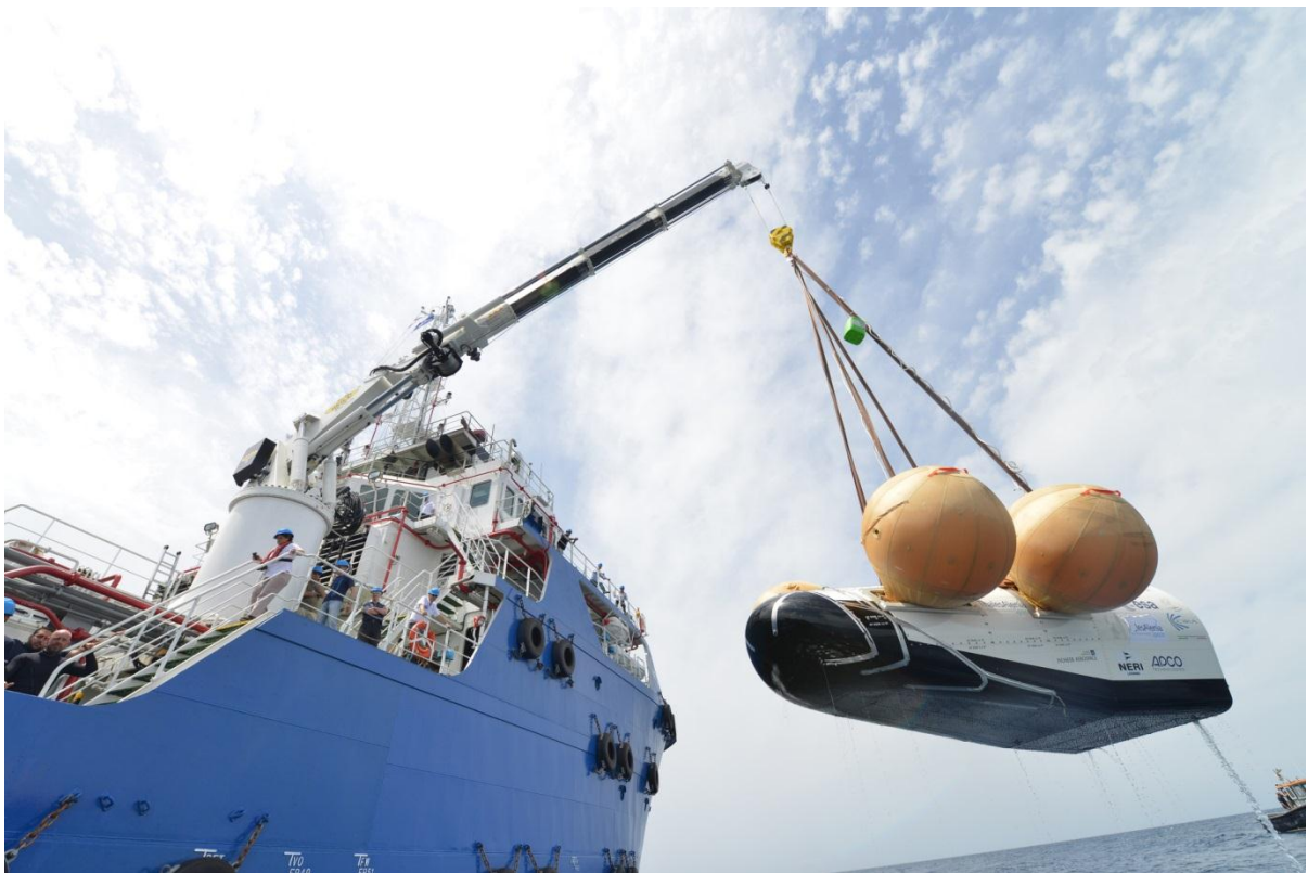
The IXV prototype is recovered and brought on board a ship during the test flight in June 2014. The orange balloons are floating devices, which inflate when the IXV touches down to ensure the IXV floats in the correct position in the water (Photograph: ESA).
