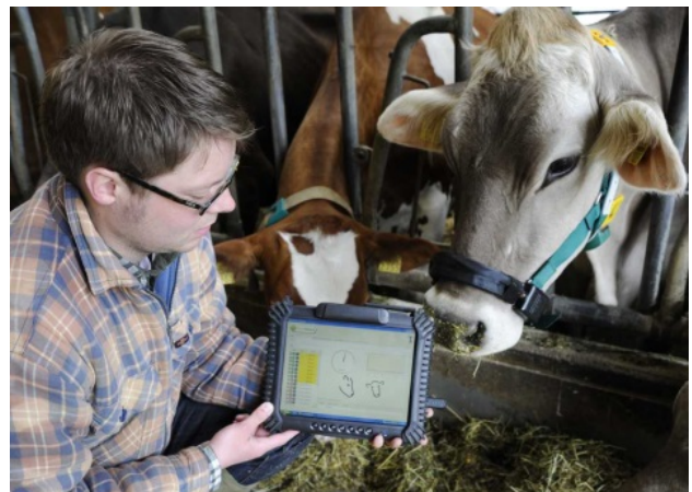
Observing chewing, ruminating, and eating patterns can tell us a great deal about a cow's health. The Rumiwatch monitoring system uses sensors to identify changes in eating patterns. (Photo: Gabriela Brändle, Agroscope)
