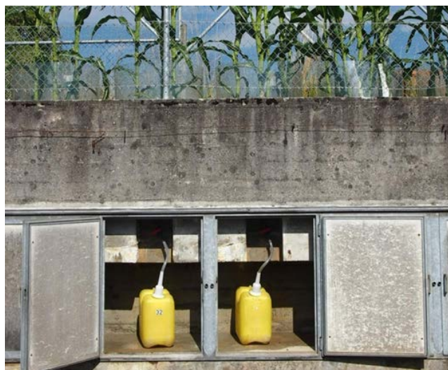
The seepage water (leachate) is collected in canisters in the maize-planted lysimeter and then analysed.
