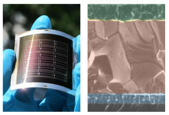
CdTe solar cells on a flexible metal foil (left) and electron microscopy (EM) image of the solar cell structure in the substrate configuration (right) with front electrical contact (uppermost layer), central CdTe layer and metal back contact (lowest layer), all deposited on the substrate (glass is used as an example for ease and clarity of EM imaging).
