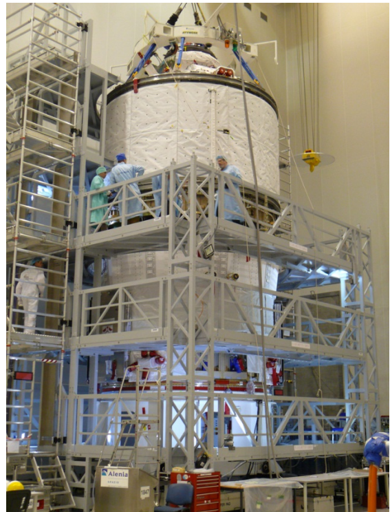
The loaded ICC (above) is lifted onto the service module (below) with the help of a crane and secured. The service module contains the propulsion engines of the ATV and supplies the satellite with electricity (Image: ESA).
