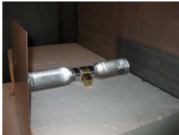
Figure 45: Measurement setup for validation of the current density probe.
