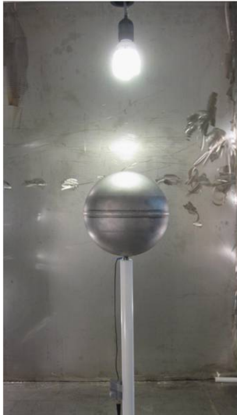
Figure 23: Test setup showing protection network connected to the Van Der Hoofden test-head, which was placed under the ESB (E4 bulb) at a separation distance of 300 mm.
