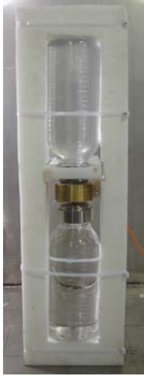
Figure 17: Linear saline phantom with current clamp (gold color). Current clamp is located between the two cylindrical bottles.
