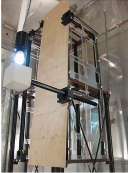
Figure 4: Measurement setup, showing the probe positioning apparatus as it positions the Narda EHP-200 probe under the light bulb.
