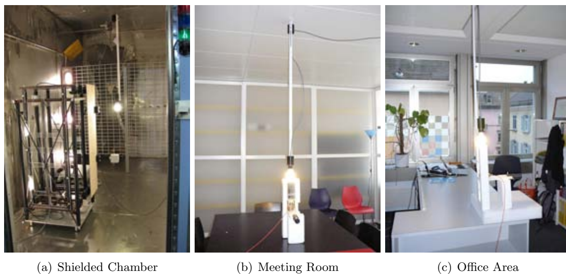
Figure 42: Bulb hanging from the ceiling is measured in different environments to test the dependance of surroundings on bulb measurements.
